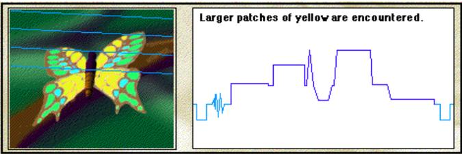
A video frame is made of lines. In NTSC there are 525 lines per frame, while PAL has 625 lines per frames. Each point in the line reflects the intensity of the video signal. At the end of each line, a horizontal sync pulse is added. This sync pulse tells the electronic devices in the CCTV
